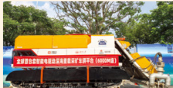
Developed the world's first 6,000-meter-class intelligent electric-drive deep-sea heavy-duty mining vehicle
